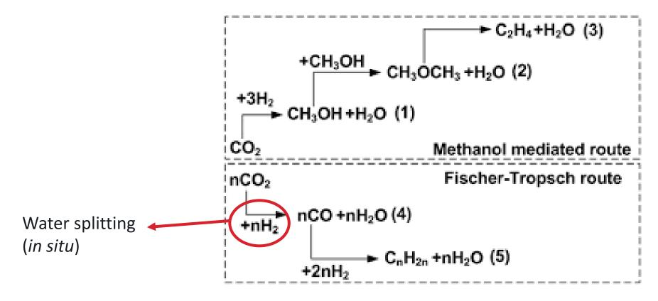
Electrolysis, photocatalysis or termal catalysis
